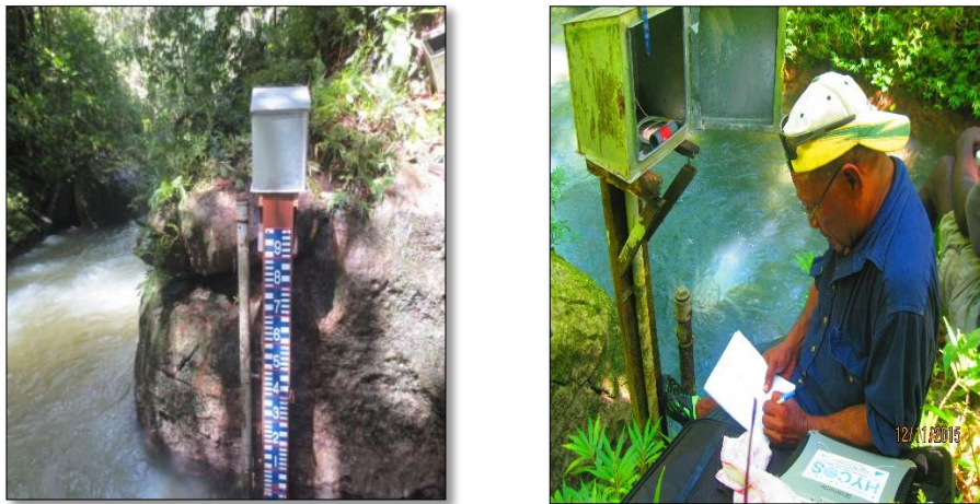
Figure 2 - Simplified Hydrological Monitoring Station
